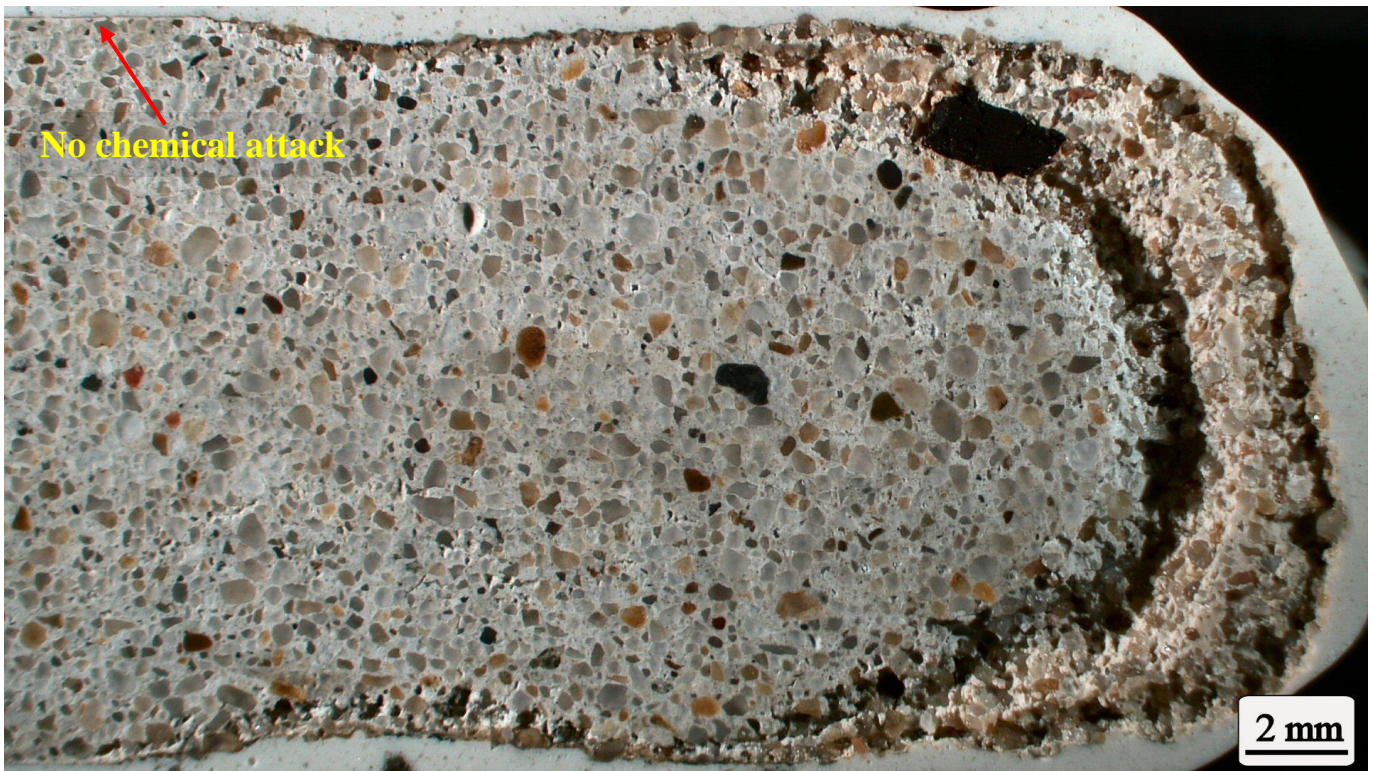
Figure 5. Cross-section photomicrographs of the grout showing the chemically attacked cement paste near the edges of the sample. Portions of the cement paste were lost during specimen preparation due to the weak nature of the material. Portions of the formed surface do not exhibit chemical attack.
