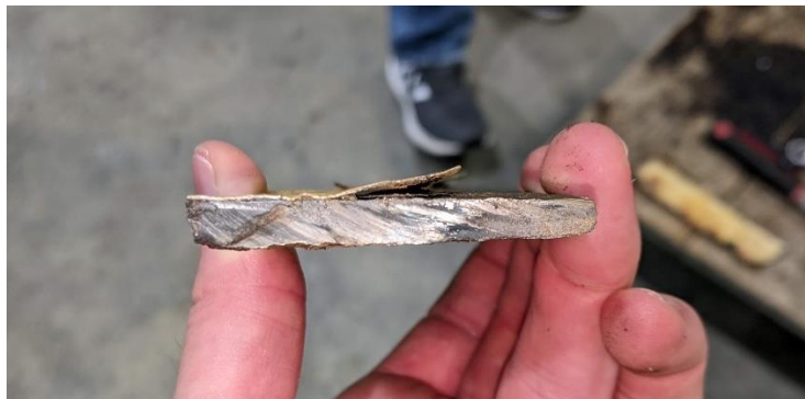
Figure 6-12: Filter 5 Bottom Flange Coupon
